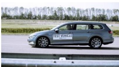
**Caption:** The car is loaded up to the permissible gross vehicle weight with two people and weights for the test. The car is brought to a standstill by braking from a speed of 100 km/h ten times in a row.
