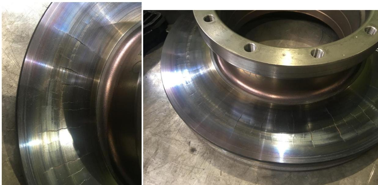
**Caption:** View of a pot side after a failed crack test
